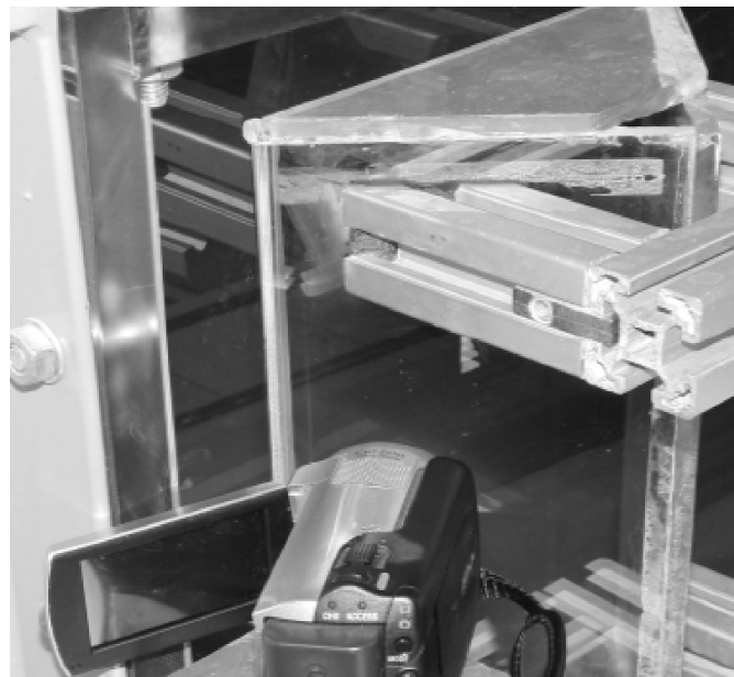
Figure 3. Picture of the prismatic window attached to the test section of the hydraulic tunnel, and the low-speed video-camera.
