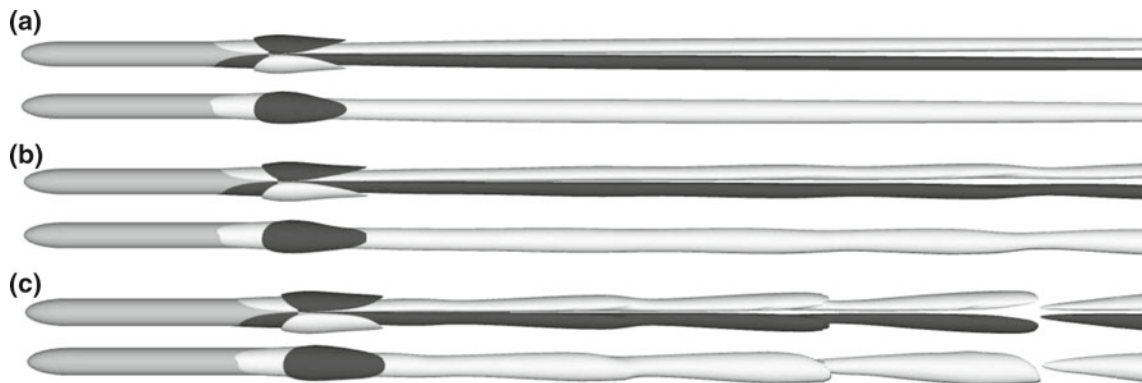
Fig. 5 As Fig. 4 for M = 0 and \omega_x = \pm 0.01 at Re = 650 (a), Re = 679 (b) and Re = 680 (c). Snapshots in subplot b clearly illustrate the 3D peristaltic instability described for the sphere wake by Gumowski et al. [11], whilst c depicts the shedding of vortices in the far wake of the solid body. See movies 1 and 2 included as supplementary material to observe the oscillatory behaviour of the afterbody wake in the absence of vortex shedding at Re = 679
