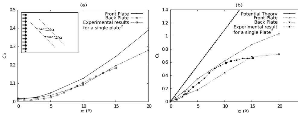
Figure 1:  $C_D$  (a) and  $C_L$  (b) as functions of  $\alpha$  for  $Re = 8 \times 10^4$ .
