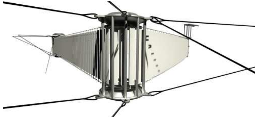
Figure 1.3: Sketch of the mooring for the tidal energy system of the Norwegian company (TidalSail S.A., 2014).
