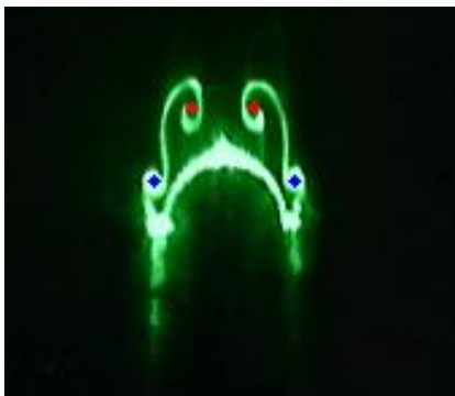
FIGURE 6. STRAKES (BLUE DOTS) AND BODY (RED DOTS) VORTEX CORES AT 27^\circ AT 5.7D
