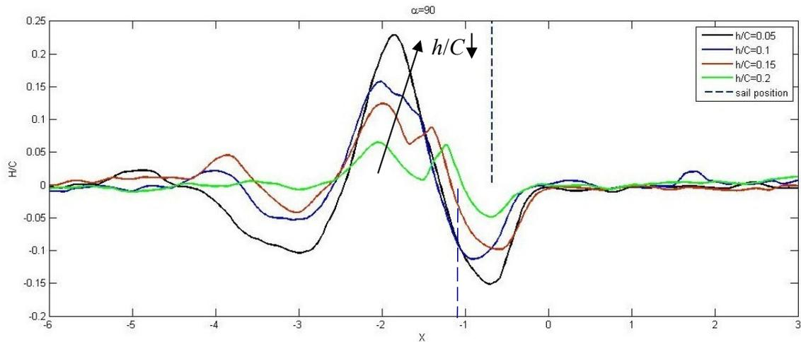
Figure 9: Non-dimensional profile of the scour for  $h/C=0.05, 0.1, 0.15$  and  $0.2$  with an angle of attack  $\alpha=90^\circ$ . The x-axis has also been made non-dimensional with the sail chord  $C$ . The flow is from right to left. The vertical dash line corresponds to the position of the sail.
