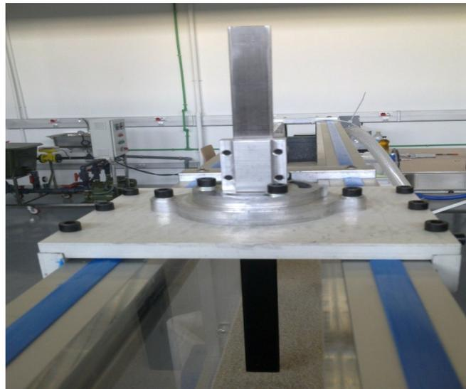
Figure 4: The sail (in black) and its support at the top of the channel of sediment.
